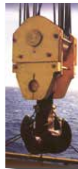
600 tonnes WLL Offshore Service Block. Quadruplex Hook
