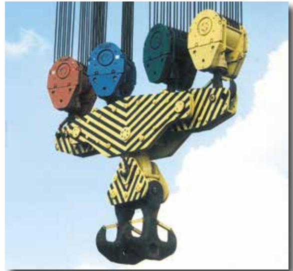
Mega Lift 3000 tonnes WLL Crane Ship Lifting System
